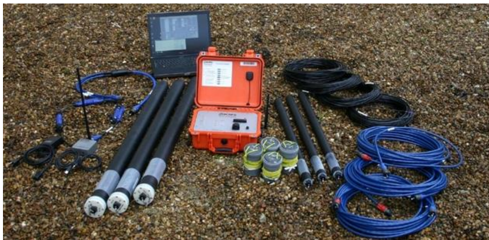
Figure 2 Top: basic schematic of MT survey layout (from seismo.geology.upatras.gr/MT.htm ); Below: Actual image of equipment- long columns are magnetometers (smaller ones not used in Rico survey), orange case is recording system, short grey and yellow columns are electrodes
