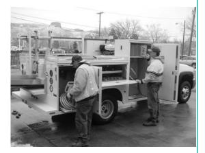
an inefficient and messy hydraulic system with a much cleaner pneumatic (air) driver for pounding sign posts into the ground. Sign installation times have been cut in half, which has additionally improved the replacement schedule. The truck also allows crews to choose between three types of pavement painting techniques depending on which application is most appropriate. The possible applications include regular: pavement painting, glued 3M tape, and thermo tape that is melted on the asphalt.
