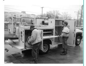
an inefficient and messy hydraulic system with a much cleaner pneumatic (air) driver for pounding sign posts into the ground. Sign installation times have been cut in half, which has additionally improved the replacement schedule. The truck also allows crews to choose between three types of pavement painting techniques depending on which application is most appropriate. The possible applications include regular: pavement painting, glued 3M tape, and thermo tape that is melted on the asphalt.
