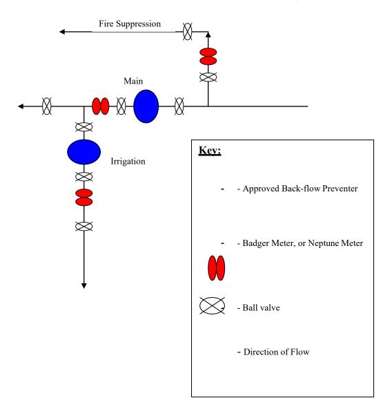
\*Note: Diagram is meant only as a guide. All plumbing fixtures shall follow International Plumbing Codes and be in accordance with State and Local Guidelines.
